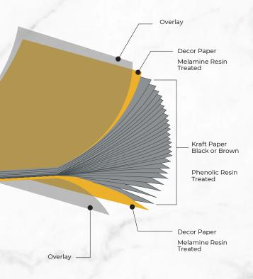
Available Thickness: 1mm to 60mm Sheet Size: 1220mm X 2440mm
